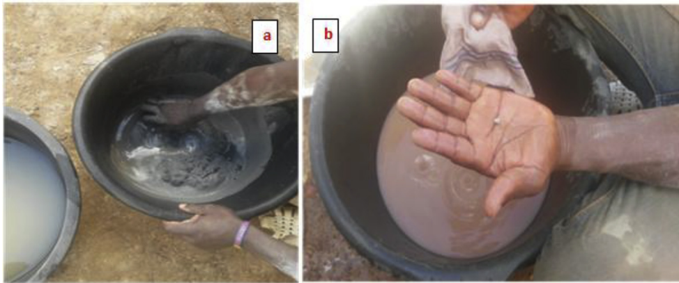
Fig. 8 – (a) Miner stirs slurry with bare hands, (b) Miner holds mercury-gold amalgam in the palm.
