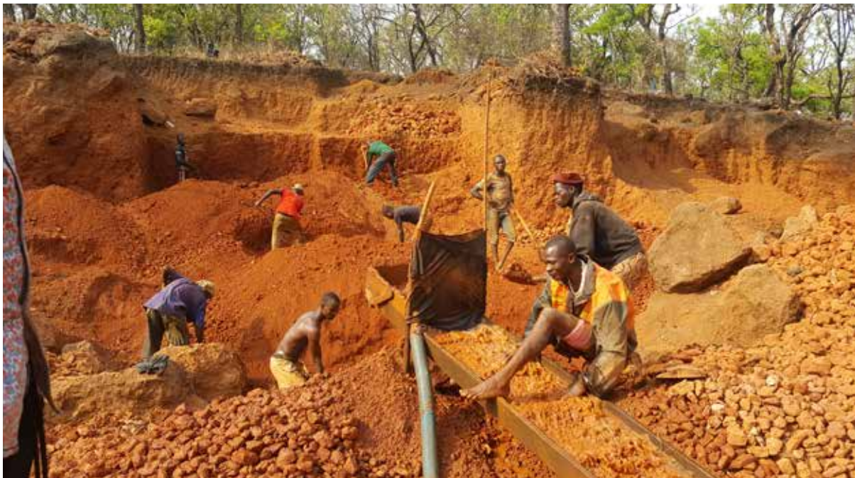
A 'gang' of 'diggers' mining and sluicing ore in Kathantha, Sierra Leone
