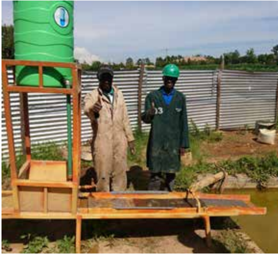
Local engineers in Mikei community, Kenya, with their reproduced MBMM sluice
