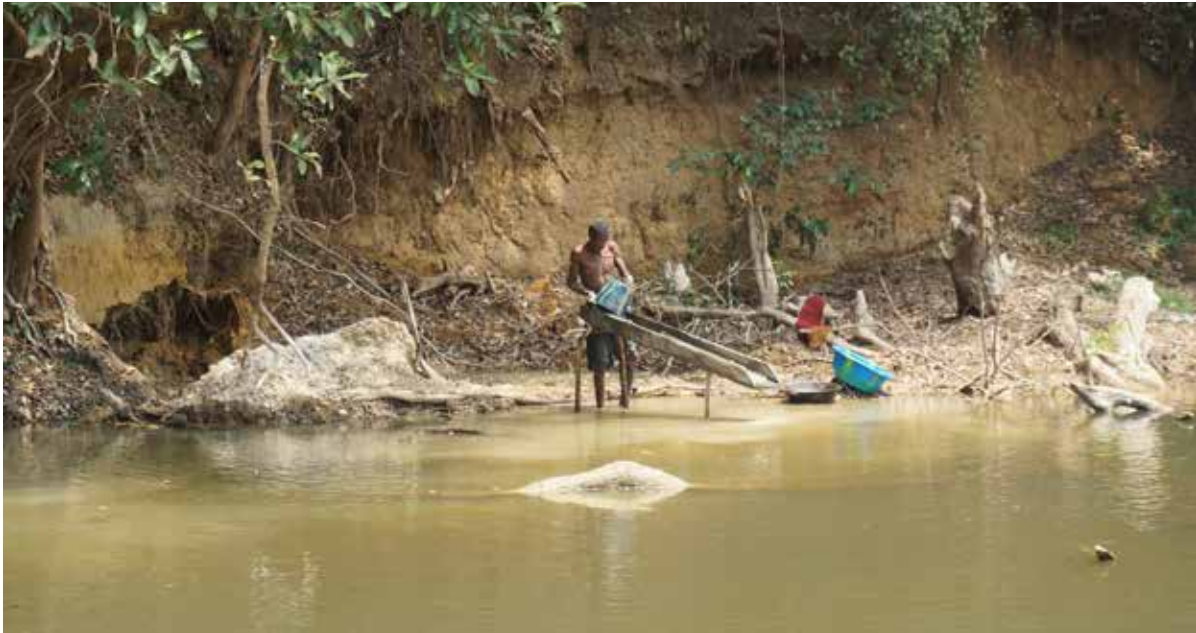
Man sluicing ore to recover gold concentrate in the Teye river, Makong, Sierra Leone
