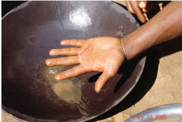
Figure 6. Mercury bead in the hands of a panner, during the process of extraction of gold by amalgamation, Hosur area, Karnataka. Note the scar on the hand of the panner.
