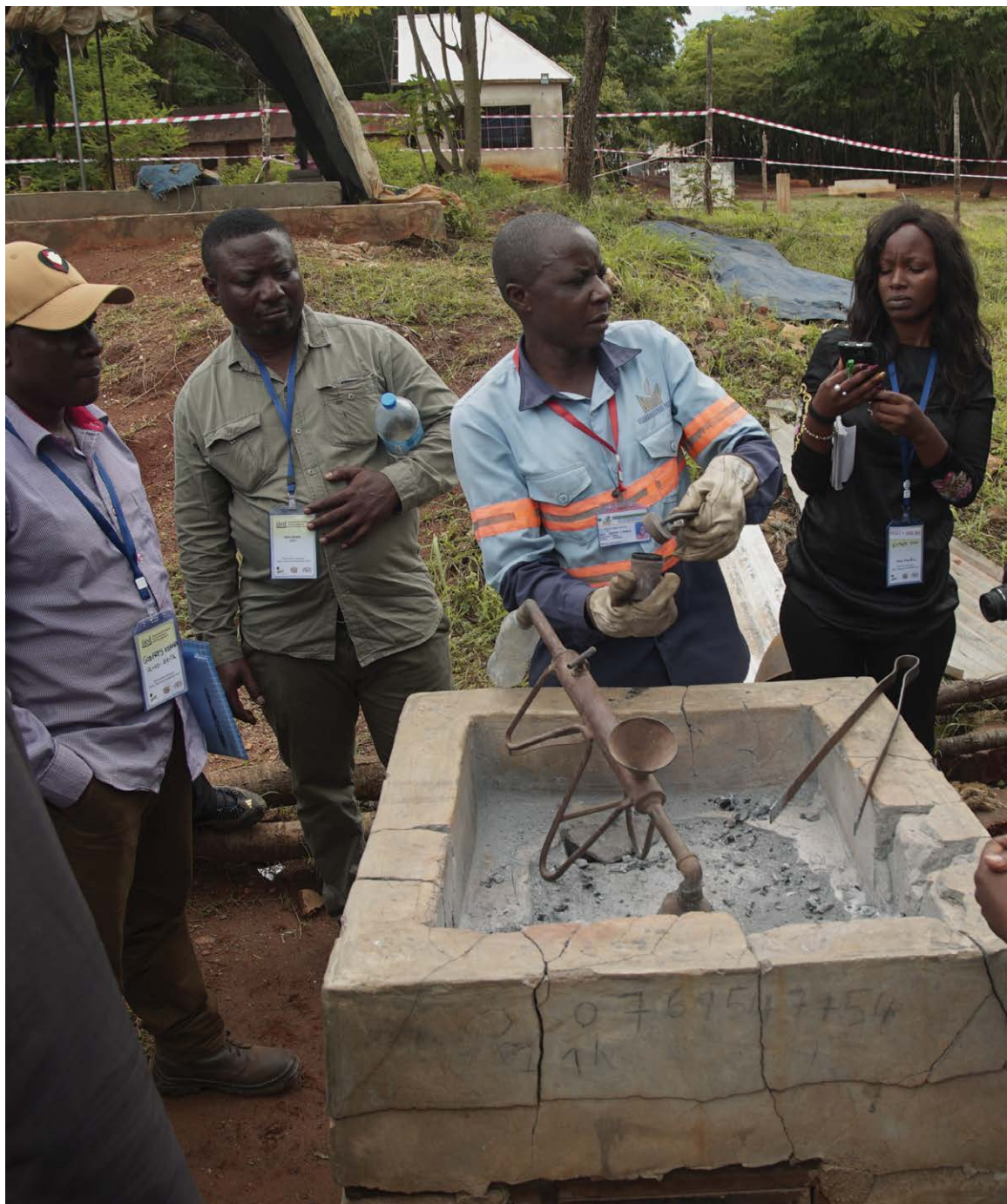
Miner demonstrating use of retort to minimise mercury pollution, Geita, Tanzania (IIED/Steve Aanu)
