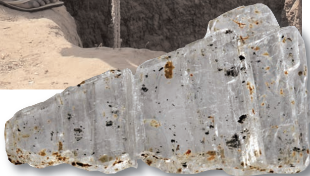
Fig. 3-9. Gypsum of the transparent type (4 cm long sample) and of the white, earthy non-transparent type next to the shaft from where it was dug out. Azara, Nasarawa State.
