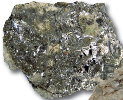
Fig. 3-6. Sphalerite (zinc mineral) with dark-brownish colour. Small amounts of galena can be seen. The yellow mineral is pyrite consisting of iron and sulphur. Sample is 15 cm long, and is from Zumo, Adamawa State.
