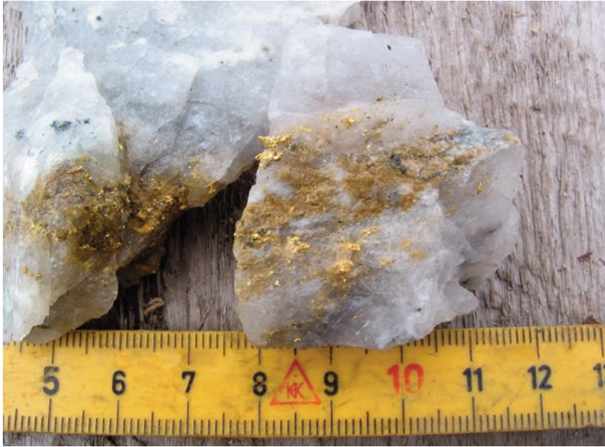
Fig. 3-4. White quartz richly mineralised with gold. Centimetre-scale for estimating size. Sample from Lasa, Borno State.
