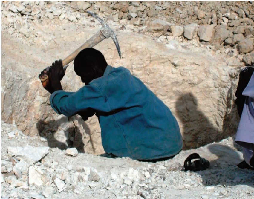
Fig. 3-11. White, very light diatomite being dug out of the ground, Alamgafi, Yobe State.
