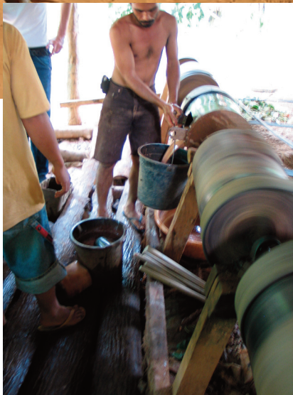
Fig. 7-1a. Dry grinding of quartz-gold ore in a ball mill produces large amounts of dust.
