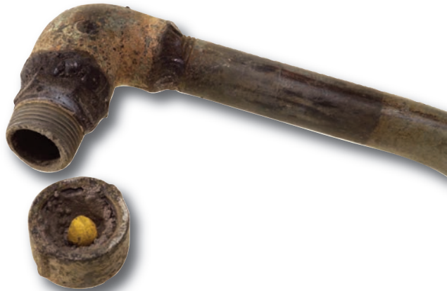
Fig. 6-5. Most of the mercury has evaporated and the gold is left behind.
