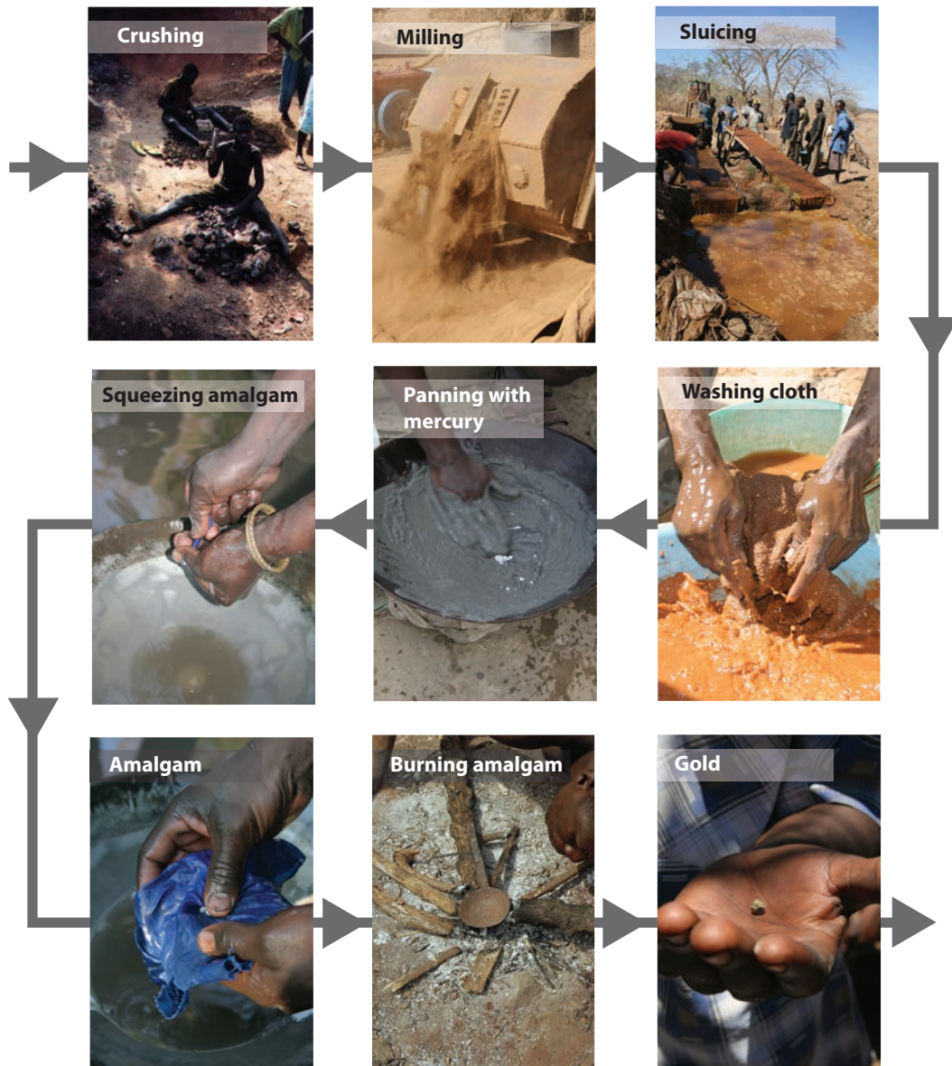
Flowchart 1. Gold extraction using mercury.
