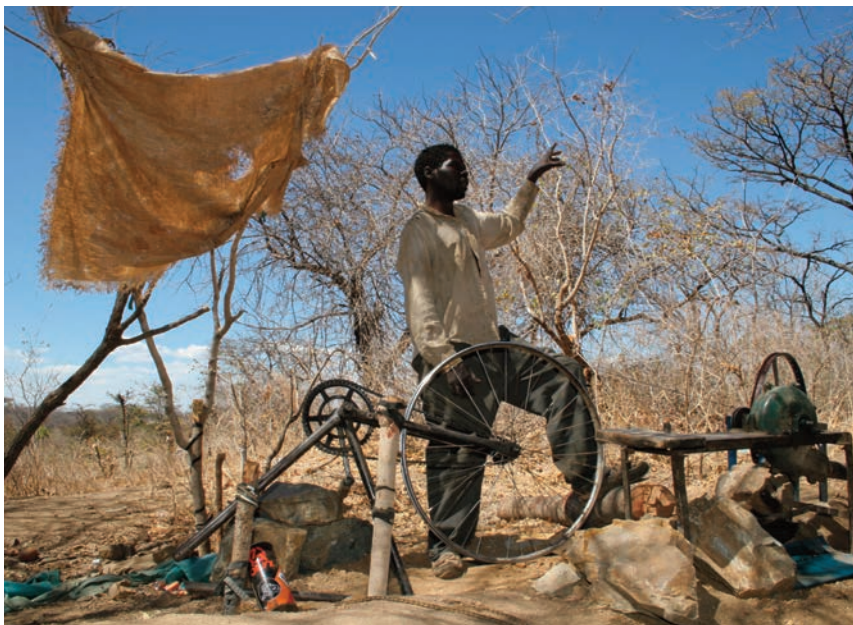
Fig. 7-12. Bicycle-powered pump for providing oxygen to tunnels.
