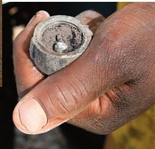
Fig. 6-3. The amalgam is placed in the cup of the retort on some ash to get the cup airtight.
