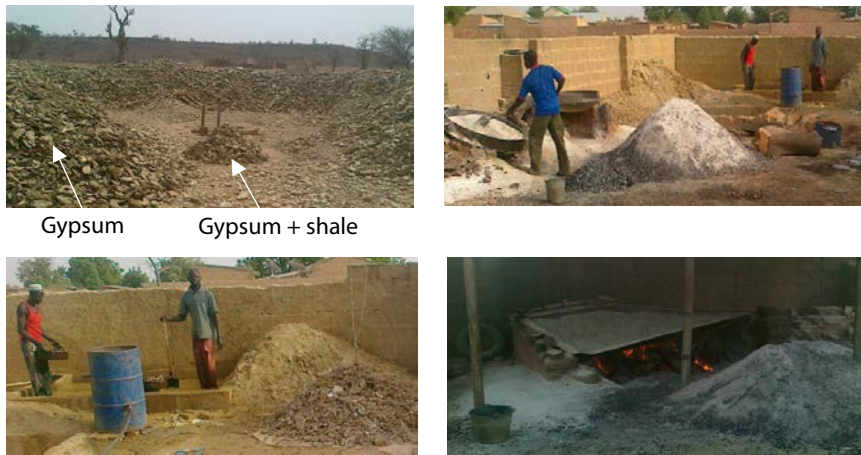
Figs 6-8 to 6-11. Gypsum pit with shale, washing and calcination by ASM operators, Yobe State.
