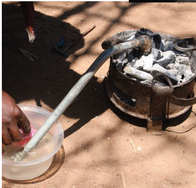
Fig. 6-4. The retort with amalgam in the cup is heated in a charcoal burner.
