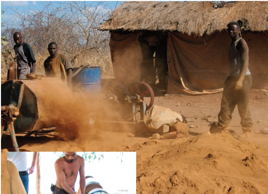
Fig. 7-1a. Dry grinding of quartz-gold ore in a ball mill produces large amounts of dust.
