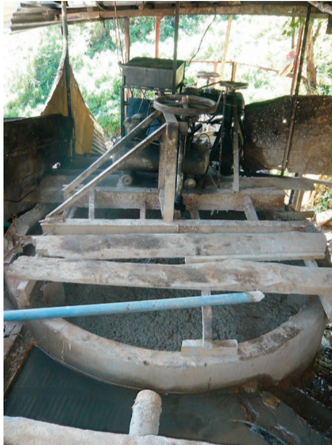
Fig. 6-7. Active leaching of tailings by cyanide. A tank containing a cyanide tailings mixture which is slowly stirred.
