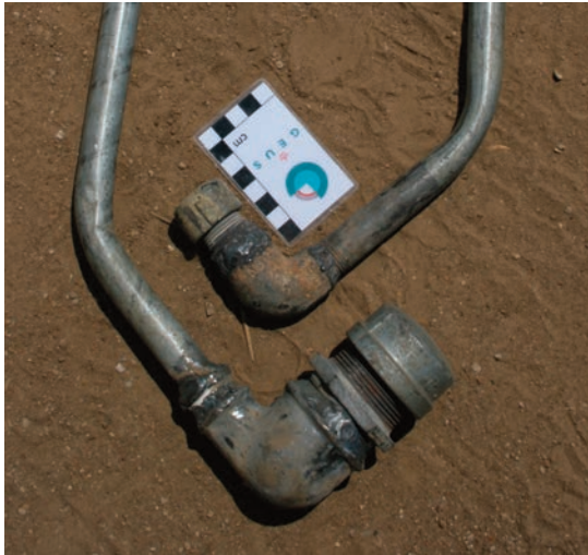
Fig. 6-2. Two retorts made of a few pieces of plumbing tubes. The scale is 10 cm.
