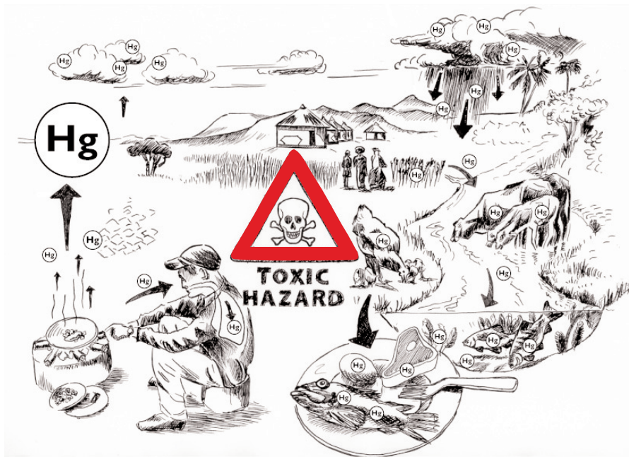
Fig. 7-3. Paths of mercury in the environment and the food chain. Hg is the chemical symbol for mercury. The 'story' starts in the lower left corner and moves forward clockwise. An ASM operator burns amalgam and thereby releases metallic mercury. He inhales some of the mercury. The rest of the mercury falls down on the soil with the rain. Then the metallic mercury is converted by bacteria to methylated mercury and enters the food chain through the drainage system and ends up in cows, hens, fish and rice. When eating the food the population is poisoned by mercury.
