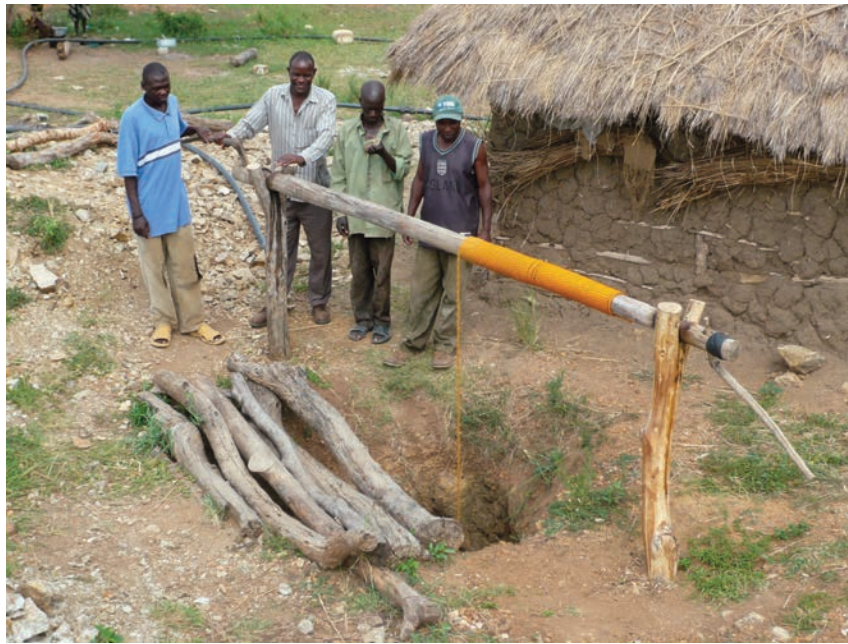
Fig. 5-6. ASM operators using a winch to raise material from a deep-shaft operation.
